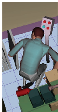
Using Jack, researchers can model human figures and investigate key ergonomic parameters in real time.
