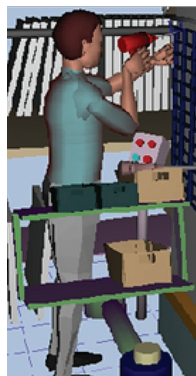
Using Jack, researchers can model human figures and investigate key ergonomic parameters in real time.
