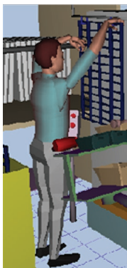
Using Jack, researchers can model human figures and investigate key ergonomic parameters in real time.
