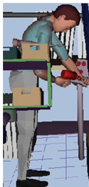
Using Jack, researchers can model human figures and investigate key ergonomic parameters in real time.
